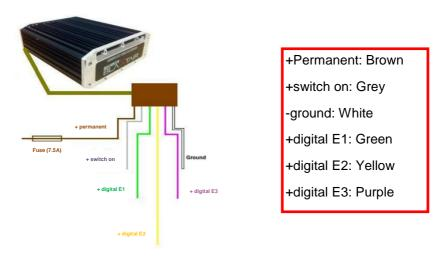
The inputs (E1, E2 and E3) are normally used for activating the detection (e.g. reverse gear). See Installation Manual.
