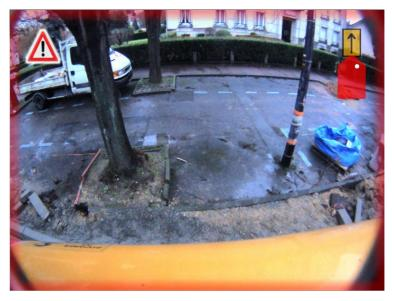
Example of obstacle detection: red frame and warning icon. In the top right corner, a radar view shows the detection zone (in red) and the approximate position of the detected obstacle (white dot).
