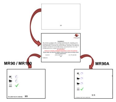
The system performs a 'self-test' sequence. Once all the ticks of this page turn green, the video is displayed on the monitor, with a green boarder, and the LED (if installed) will turn green indicating that Blaxtair system is now fully operational.
