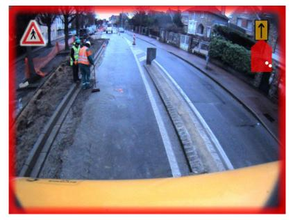
Example of pedestrian detection: red frame and pedestrian icon. In the top right corner, a radar view presents the detection zone (in red) and the approximate position of the detected pedestrians (white dots).
