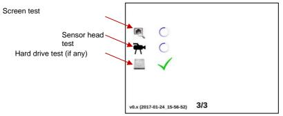
Do not shut down the processing unit during initialisation. The complete initialisation process can last from 30 to 70 seconds.
