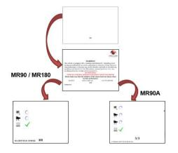
The system creates a self-diagnostic sequence. Once all the items on this page have received a green tick, the video is displayed on the screen with a green frame and the LED (if installed) turns green, indicating that the Blaxtair system is now fully operational.
